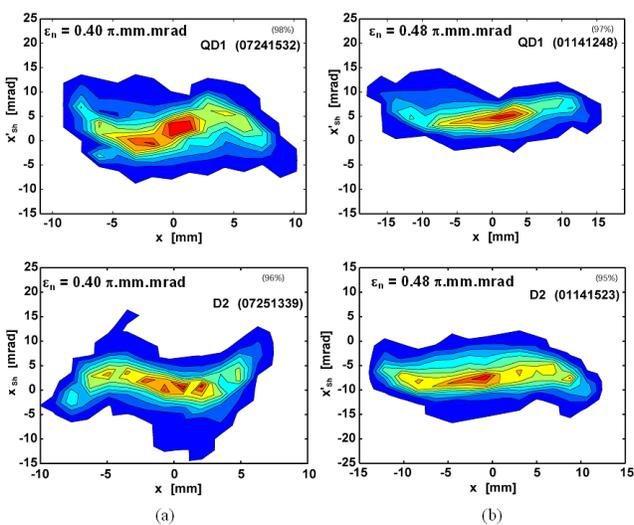
**Figure: Horizontal phase-space diagrams measured before (top) and after (bottom) the electrostatic transport section for (a) 60% fill factor; (b) 80% fill factor, for a single time slice at mid-pulse.**
