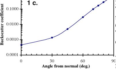
**Fig. 1. (a) Measured electron emission coefficient, and (b) Gas desorption coefficient; (c) Ion backscatter from a smooth surface, as predicted**
