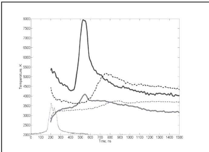
**Figure 3:** Figure 3: Pyrometer record comparing solid (solid lines) and porous (dashed lines) gold foils. Porous samples are 35% of solid density. Lower solid grey line- brightness temperatures at 900 nm, fitted, lower left: dotted line-temporal profile of heating beam in arbitrary units.
