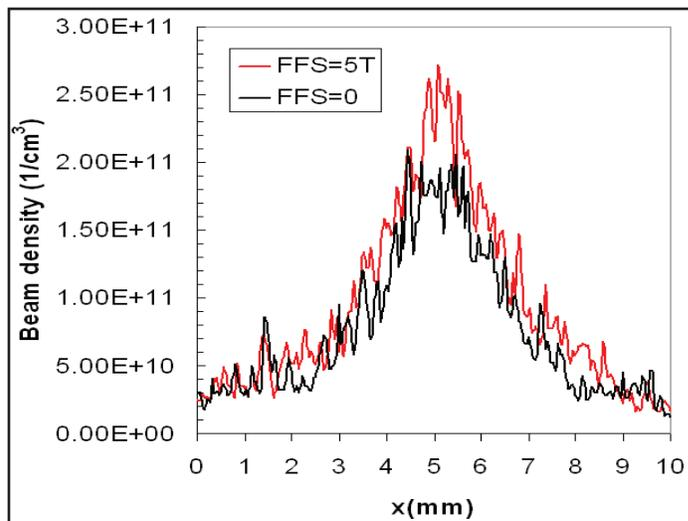
**Figure 2:** Beam density profiles at the target focal plane with the final focus solenoid on (FFS=5T) and off (FFS=0). The corresponding focal spot FWHM = 2 mm with FFS=5T and 3 mm with FFS=0.
