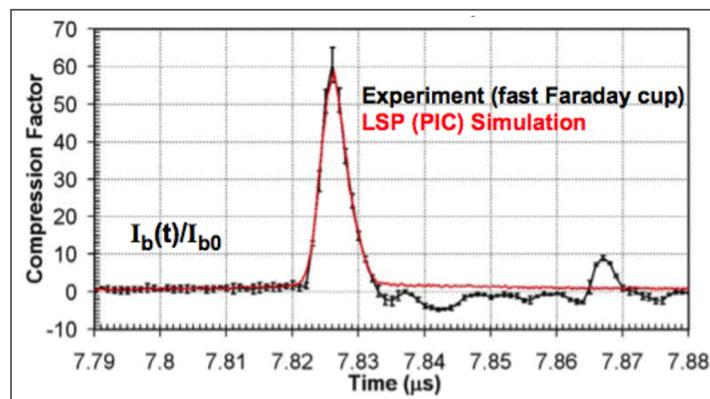
**Figure 2.** Comparison of fast Faraday cup current waveform with LSP PIC simulations for NDCX compression experiment. When the actual, experimentally realized waveforms were inserted in the simulations, good agreement with the data was obtained.
