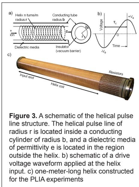
**Figure 3.** A schematic of the helical pulse line structure. The helical pulse line of radius  $r$  is located inside a conducting cylinder of radius  $b$ , and a dielectric media of permittivity  $\epsilon$  is located in the region outside the helix. b) schematic of a drive voltage waveform applied at the helix input. c) one-meter-long helix constructed for the PLIA experiments
