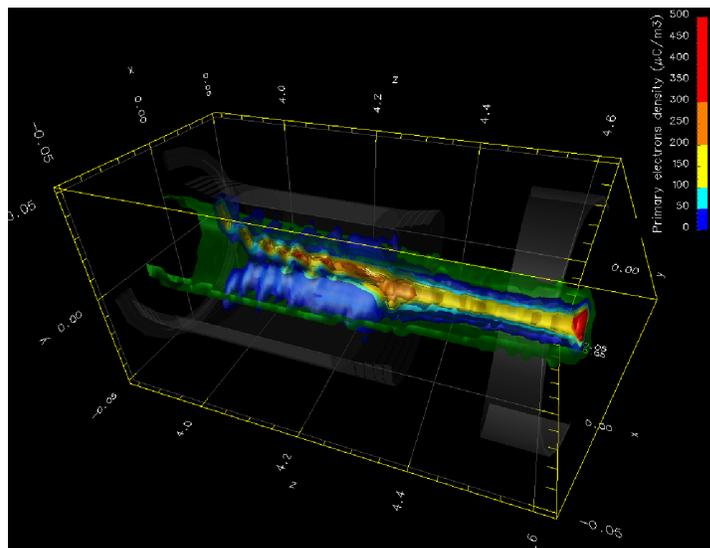
**Figure 4.** The charge density of primary electrons (color coded) are simulated from emission off the beam hitting the end wall on the right, and extending from through the last magnet to the clearing electrode between the last two magnets.
