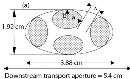
**Figure 2** – Schematic of the beam footprints at the exit of QD5. The individual beams size is  $a=3.7 \times b=3.7$  mm. The beam-edge to beam-edge clearance is  $\Delta = 4$  mm.
