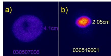
**FIG. 1.** Beam images for a 255 keV beam measured 1m downstream as transported through a tube of diameter (a) 15 cm and (b) 7.6 cm.
