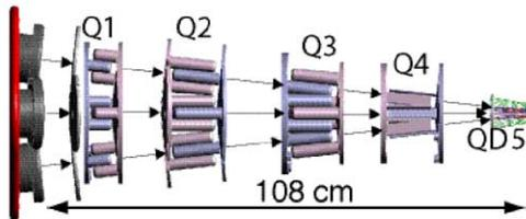
**Figure 1** – A CAD view of the lattice elements of the Combiner apparatus. The first four elements (Q1-Q4) are electrostatic quadrupoles. QD5 is the combined function dipole and quadrupole, for which the electrostatic field-defining rods around each beam converge as  $z$  increases.
