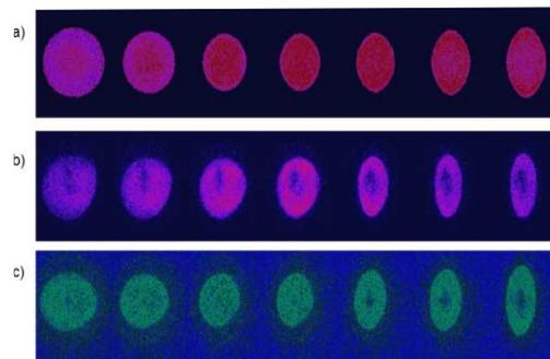
**FIG. 2.** Vacuum transport beam profile for 240-310 keV energies in (a) WARP calculations, (b) for transport through a 15 cm diameter tube and (c) for transport through a 7.6 cm diameter tube using the biased mesh.
